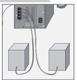
1 Connect the loudspeaker cables to the »SPEAKER R +/-L +/-« terminals on the hi-fi system and the »- INPUT +« terminals on the loudspeakers. Connect the cables marked to the red terminal.
